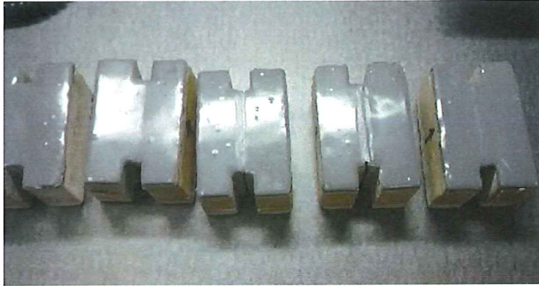
After 10 cycles Tecnocoat P-2049 – no crack
