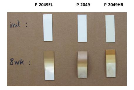
It is not recommended to use the above Tecnocoat polyurea systems as **primary lining** material in storage tanks for crude oil.
